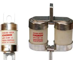
**BS 88 Extremely high breaking capacity fuses:** protection of power semiconductors as per IEC Standard 60269.1 and 4 690 V voltage rating aR (ratings from 6 to 710 A) as per UL and IEC 60269.4
