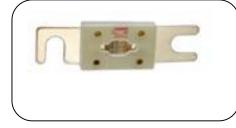
Forklift truck and battery isolator fuses are specially designed for the heavy duty loads associated with DC battery powered equipment such as forklift trucks, hand trucks, motorized work platforms, and other DC battery operated systems. stud mounted bolt-in design assure a long life in adverse conditions for these fuses. 35A to 800A, IEC 60269 CE
